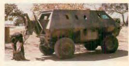
Above: Side view of Bullet. Note firing ports. Carries crew of 10. Vehicle commander leads squad when they dismount. Production version will mount .30 or .50 cal MGs or 20mm cannon.
